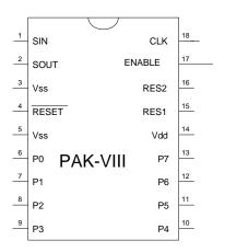
The PAK-VIII is a standard 18-pin IC. In order to operate, it must have a regulated supply of 5V and connection to a clock element. The PAK-VIII includes a 50MHz ceramic resonator that you can use to clock the chip. If you need more accuracy, a crystal or external oscillator may be used.
