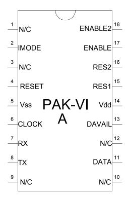
WARNING: The PAK VIa is a static-sensitive, CMOS device. Observe static precautions when handling. Operating the device without both Vss pins grounded or with RES1 or RES2 disconnected may damage the chip.
