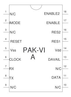
WARNING: The PAK VIa is a static-sensitive, CMOS device. Observe static precautions when handling. Operating the device without both Vss pins grounded or with RES1 or RES2 disconnected may damage the chip.
