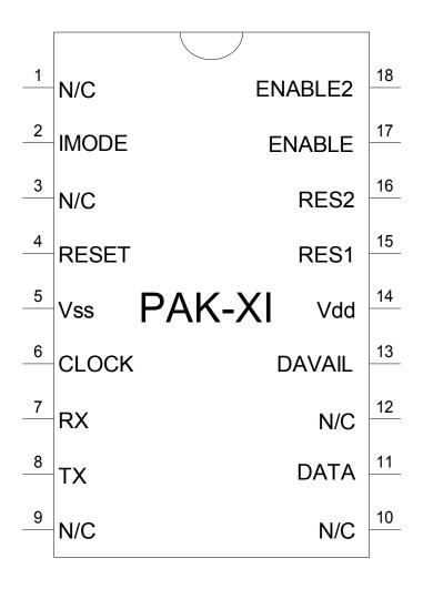
WARNING: The PAK XI is a static-sensitive, CMOS device. Observe static precautions when handling. Operating the device without both Vss pins grounded or with RES1 or RES2 disconnected may damage the chip.
