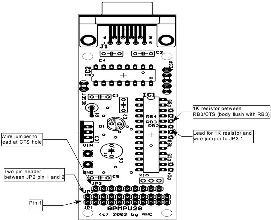
Figure 2. GPMPU28 Modifications
